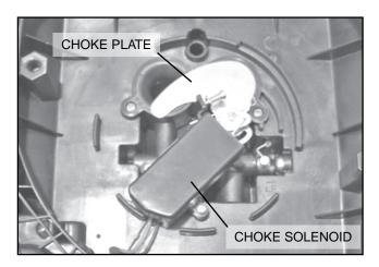
Figure 22. Solenoid De-Energized, Choke Closed 12-20 kW Units
